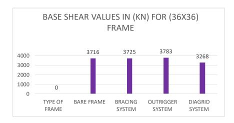
Fig. 14. Base shear values (in KN) for (36x36 Frame).
