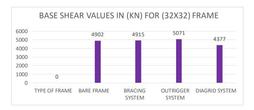
Fig. 13. Base shear values (in KN) for (32x32 Frame)
