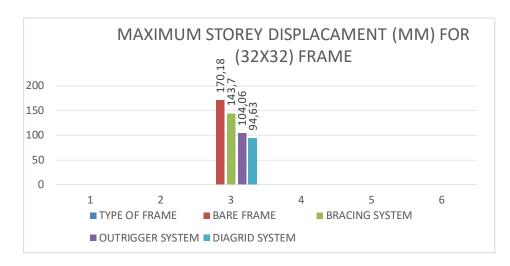
Fig. 7. Maximum Storey Displacement (in mm) for (32x32) Frame.
