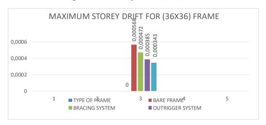
Fig. 11. Maximum Storey Drift for (36x36) Frame.
