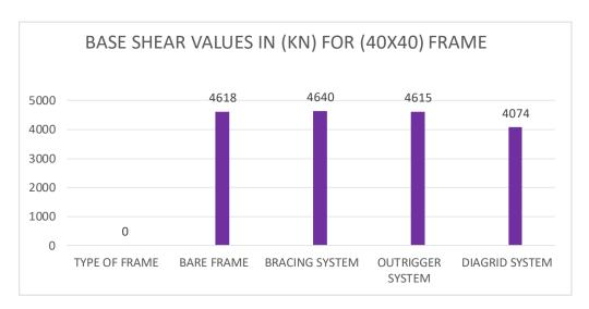
Fig. 15. Base shear values (in KN) for (40x40 Frame).
