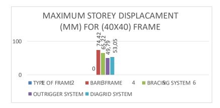
Fig. 9. Maximum Storey Displacement (in mm) for (40x40) Frame.
