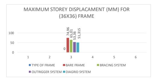
Fig. 8. Maximum Storey Displacement (in mm) for (36x36) Frame.
